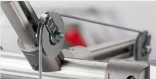
Cables often need to be redirected to create compact and efficient constructions. The Cable Pulley Wheel D42/D6-12 offers simple and secure guidance for cables. This high-quality, ball-bearing pulley can be screwed directly to the profile with or without Spacer Bushings. The bracket plate included in the scope of supply stops the cable from springing out of the pulley.
