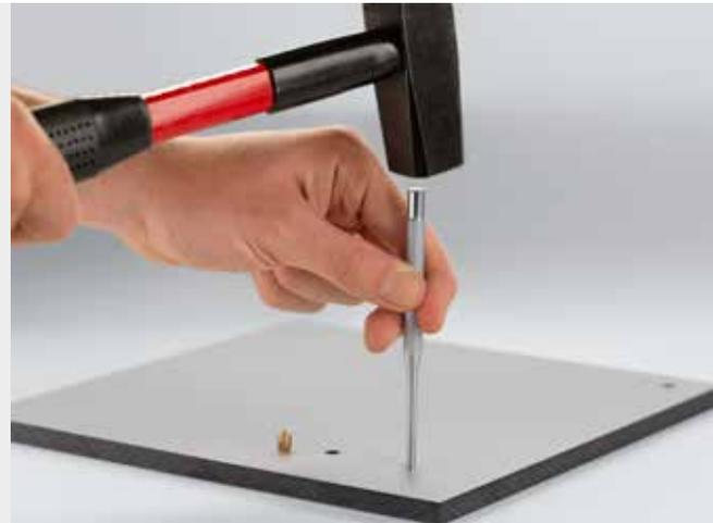
Inside Expansion Insert M5x8 is a special spreader plate. When installing the Insert in a predrilled hole, a number 3 pin punch can be used to force this plate down, thereby firmly anchoring the serrated edge in the workpiece.
