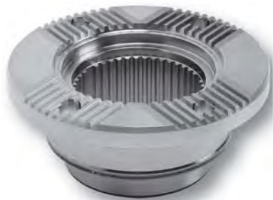
Design according to DIN ISO 8667 – Induction-hardened and lead-free ground seal bearing surface – Internal splines – Cross-serration 70°
