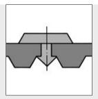
Proximity-Switch Cam 8 is pressed into the flat side of the Timing Belt at the required positions.
