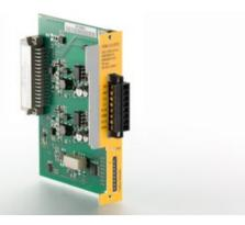
Safety Module STO (Safe Torque Off) is an expansion add-on for item Controllers in the C series. It ensures that, when at rest, the Motor does not produce any effective torque. This means the system is shut down safely when, for example, the emergency shutdown button is pressed or a door is opened.
