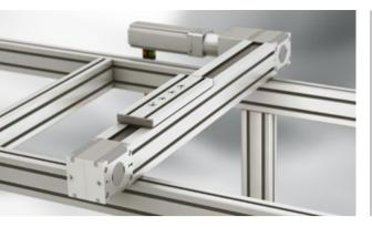
Everything in one housing. The roller elements of the compact item Linear Units KLE run inside the profile. With the exception of the carriage, none of the moving parts can be touched because the timing belt in the guide groove covers the moving elements. This enhances occupational health and safety and reduces soiling on the guides and roller elements.
