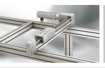
Thanks to its criss-crossed roller guide and high-strength steel tracks, Linear Unit KRF is ideal for demanding applications. Two Linear Units KRF can work in parallel via a synchronous drive, with Linear Unit KRF 8 80x40 ZR, synchronous drive responsible for guidance. As the shaft on the drive side passes straight through, a synchroniser shaft can be connected to it. Synchronising Set KRF 8 80 ZR (0.0.648.58) is used to make this connection.
