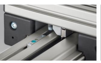
Always know your limits! item Proximity Switches are used for homing and for identifying the end positions on Linear Units. They are inductive devices and send their signals to the Controller via a connecting cable.
