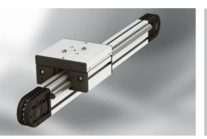
Linear Unit LRE 8 D14 80x40 KU 80 is secure and virtually indestructible. The 1/2" roller chain delivers consistently high power transmission and a reliable hold when used in vertical applications. Even very heavy loads up to 1600 N are moved in a controlled manner and with powerful acceleration. Linear Unit LRE 8 D14 80x40 KU 80 can also be used in heavily contaminated environments.
