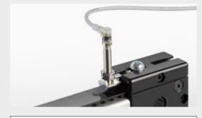
The Proximity-Switch Fastening Set is used to position and attach inductive Proximity Switches M8 on the Timing-Belt Reverse Units. Proximity-Switch Connecting Cable in plug-in design with integrated LEDs for displaying the switch function and operating voltage.
