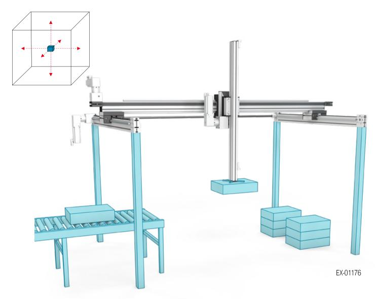
3D gantries carry out demanding positioning tasks in three dimensions. They are used to pick up, move and set down workpieces for stacking, sorting and machining operations. When designing pick-and-place systems, it is important, on the one hand, that the right grippers and tools for the task can be attached. On the other hand, the rigidity of the overall construction is crucial. This prevents load-related vibration on the Z axis and thus enhances the gantry's precision.
