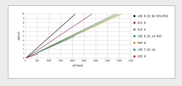
Travel speed v in relation to input speed n (ball screw, chain and rack drives)
