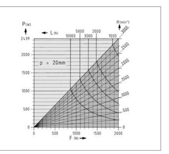
The maximum travelling speed of the spindle units depends on the length of the spindle (see adjacent diagram).
