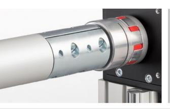
Connecting Shafts are used to provide a torsionally rigid connection between the mechanical drive elements and the corresponding Coupling Half. The Connecting Shafts are inserted into the drive elements until they come up against the stop of the Snap Ring. The clampable Coupling Half is slipped onto the free end of the shaft and clamped axially such that the length of the coupling matches the length of the Coupling Housing, and the Coupling Inserts are not under any axial load.
