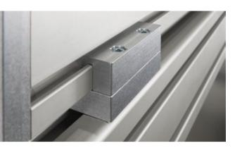
Profile Fastening Set 6/8 80x60 creates a friction-based con-nection between a component that has a Line 6 groove on its side and a base that features a Line 8 groove. This means, for example, that a 60 mm-wide Linear Unit can be fastened to a Line 8 support profile. The installation process is very easy and the shape of the fastener means that the components centre themselves.
