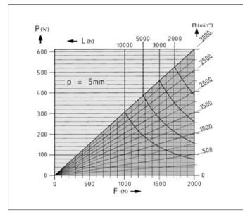
The service life of the screw and drive nut combination can be calculated based on the thrust load and drive speeds
