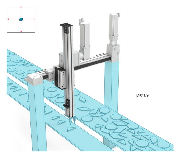
Grippers, suction cups, lasers and scanners are used in XY tables for machining, sorting, positioning and inspecting workpieces. The tool is often guided into place from above via a cantilever axis, while the X axis is used to move it to different positions. 2D linear gantries are perfect for dynamic pick-and-place tasks. Unlike 2D flat gantries, the working area of the tool can be adapted to the contour of the workpiece.
