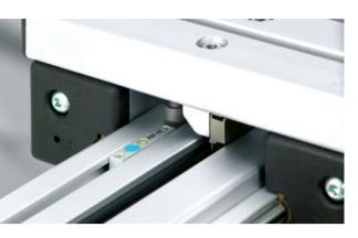
Proximity Switch M8 is a versatile device for limiting the terminal position or for reference on Linear Units with timing-belt drives. It is available with a permanent or plug-in connecting cable.
