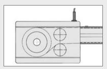
When using a system that reverses the timing belt via contact with its flat side (Timing-Belt Counter-Reverse Unit 8 R25/ Timing-Belt Reverse Unit 8 80 R25 with emergence 40 mm), Proximity-Switch Cams 8 must not pass through the Timing-Belt Reverse Units. In this case, Proximity Switches 8 and Proximity-Switch Cams 8 must be positioned to prevent this from happening.
