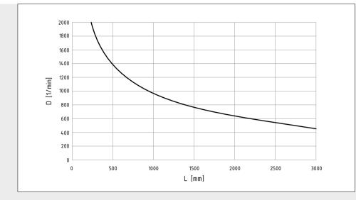
0.0.463.56 Synchronising Shaft Profile VK32 D = speed [RPM] L = length of shaft [mm]
