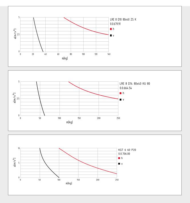
h = horizontal orientation v = vertical orientation
