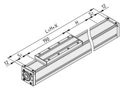
Linear Unit KGT 6 60 P20 2600 Maximum stroke H<sub>max</sub> mm Mass per mm of stroke  $m_2$ Total mass m =  $4.2 g/mm m_1 + H * m_2$ Repeatability Maximum acceleration 0.01 mm 15 m/s<sup>2</sup> Maximum travelling speed 1 m/s Feed constant 20 mm/r 1 pce. 0.0.706.00
