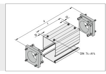
The conduit elements are fixed in place between the two drive units of Linear Units KRF using the adapter plates in the Synchroniser Shaft Cover Set.
