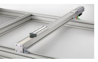
Linear Unit KGT 6 60 P20 combines a ball screw drive that has a stroke of up to 2600 mm with a strong carriage, and does so in the smallest of installation spaces.
