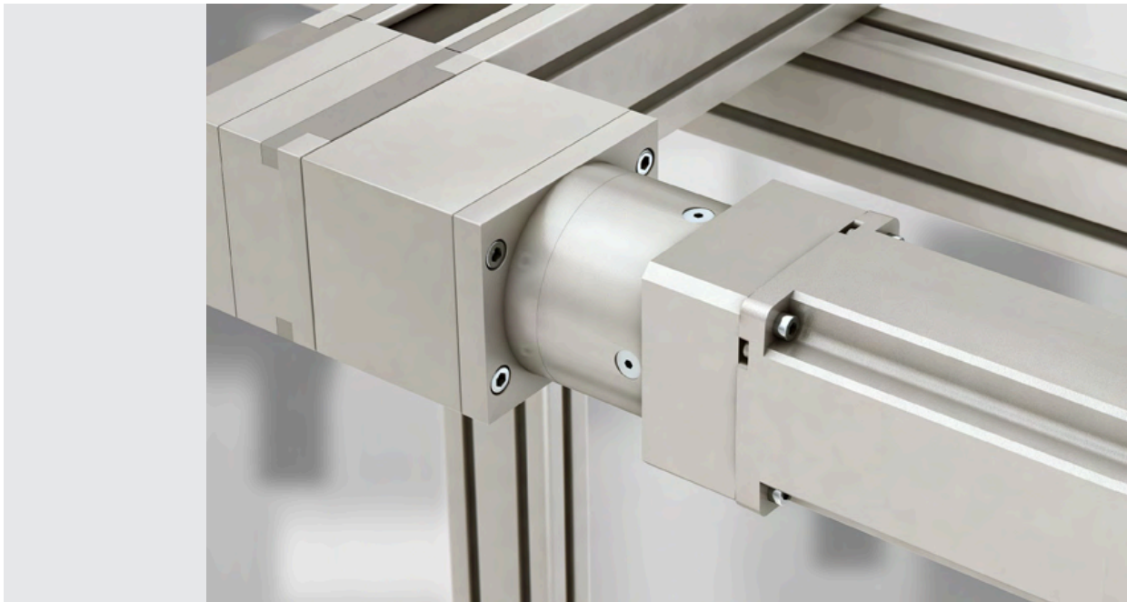
To achieve the desired torque, the motor here (right) is connected via a compact planetary gearbox. The drive shaft continues to run thereafter into the drive of the linear unit (left).
