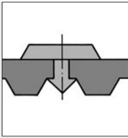
Proximity-Switch Cam 8 is pressed into the flat side of the Timing Belt at the required positions.
