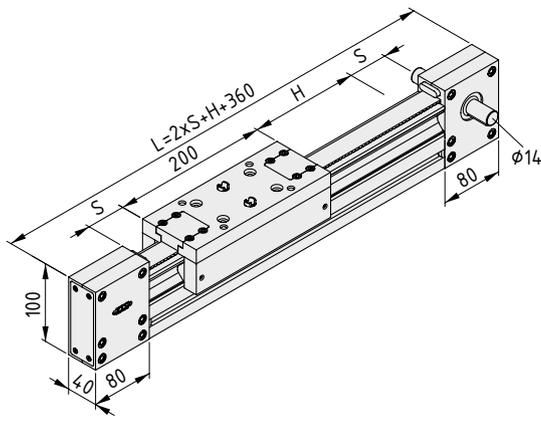
**Linear Unit KRF 8 80x40 ZR, synchronous drive**
