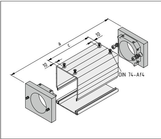
The conduit elements are fixed in place between the two timing-belt drives of Linear Units KLE using the adapter plates in the Synchroniser Shaft Cover Set.
