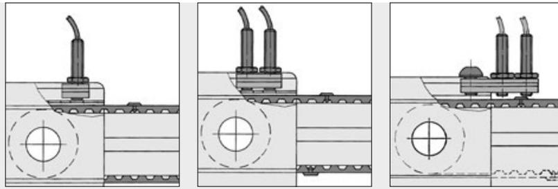
Options for installing Proximity Switches 8 using the Proximity-Switch Fastening Set. Depending on the application, the Proximity-Switch Fastening Set must be shortened accordingly.
