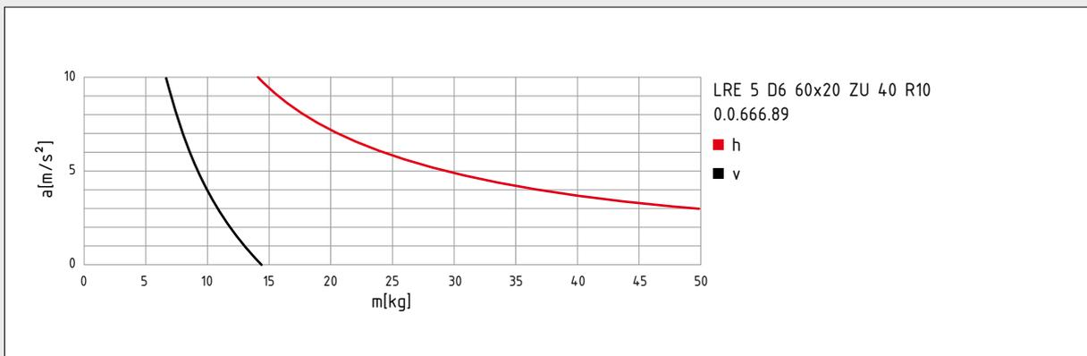
h = horizontal orientation    v = vertical orientation
