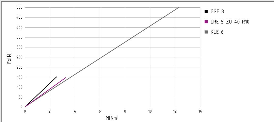
Operational force  $F_x$  dependent on input torque  $M$  (ball screw drive, chain drive, rack drive)
