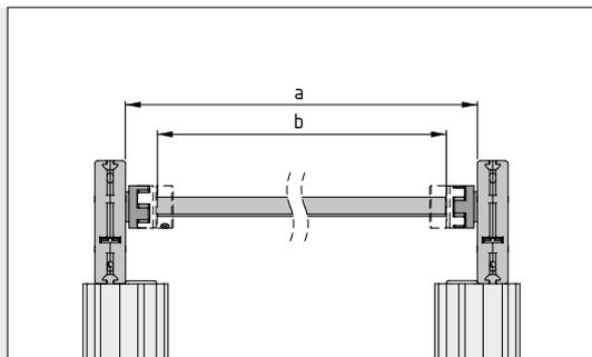
A suitable Tube St (sawn to length) turns the Synchronising Set into a complete synchroniser shaft.
