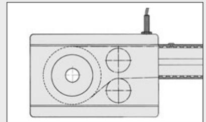
When using a system that reverses the timing belt via contact with its flat side (Timing-Belt Counter-Reverse Unit 8 R25/ Timing-Belt Reverse Unit 8 80 R25 with emergence 40 mm), Proximity-Switch Cams 8 must not pass through the Timing-Belt Reverse Units. In this case, Proximity Switches 8 and Proximity-Switch Cams 8 must be positioned to prevent this from happening.
