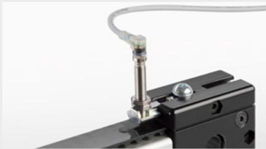
The Proximity-Switch Fastening Set is used to position and attach inductive Proximity Switches M8 on the Timing-Belt Reverse Units.
