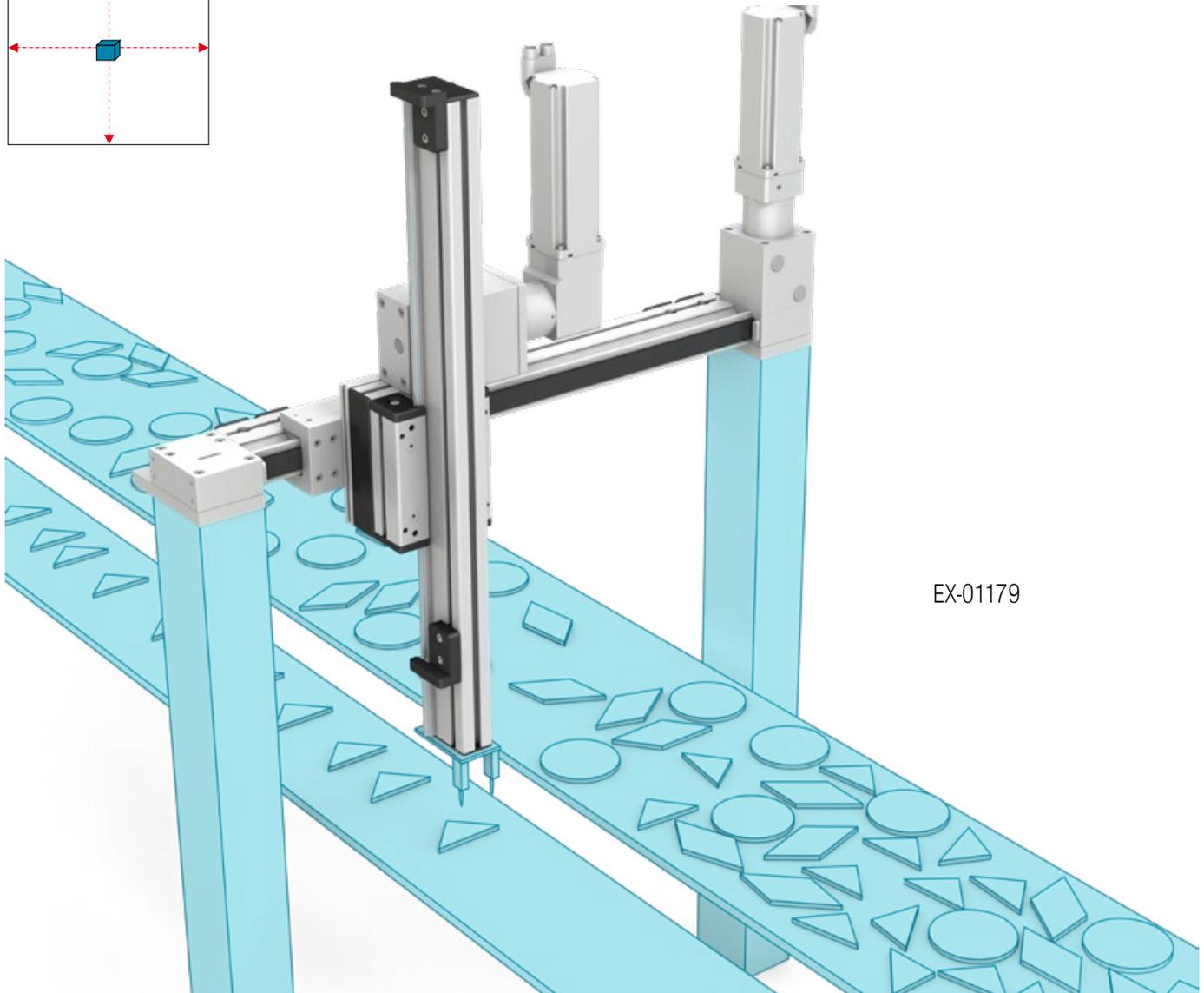
Grippers, suction cups, lasers and scanners are used in XY tables for machining, sorting, positioning and inspecting workpieces. The tool is often guided into place from above via a cantilever axis, while the X axis is used to move it to different positions. 2D linear gantries are perfect for dynamic pick-and-place tasks. Unlike 2D flat gantries, the working area of the tool can be adapted to the contour of the workpiece.
