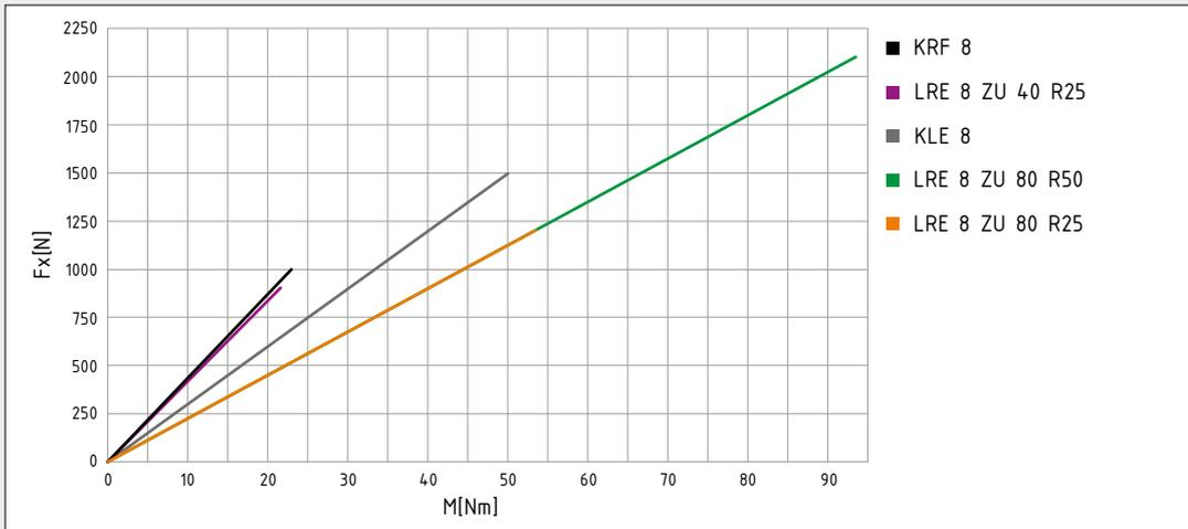
Operational force  $F_x$  dependent on input torque  $M$  (timing-belt drives  $F_x \leq 500N$ )
