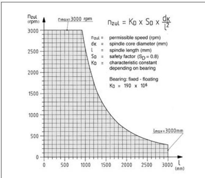
The maximum travelling speed of the spindle units depends on the length of the spindle (see adjacent diagram).
