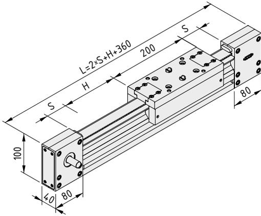
**Linear Unit KRF 8 80x40 ZR, right-hand input shaft**
