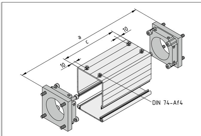
The conduit elements are fixed in place between the two drive units of Linear Units KRF using the adapter plates in the Synchroniser Shaft Cover Set.
