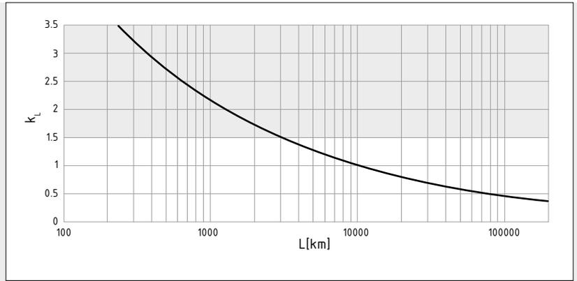
$$k_L = \frac{|M_x|}{M_{x \max}} + \frac{|M_y|}{M_{y \max}} + \frac{|M_z|}{M_{z \max}} + \frac{|F_y|}{F_{y \max}} + \frac{|F_z|}{F_{z \max}}$$
