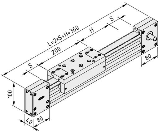
**Linear Unit KRF 8 80x40 ZR, left-hand input shaft**
