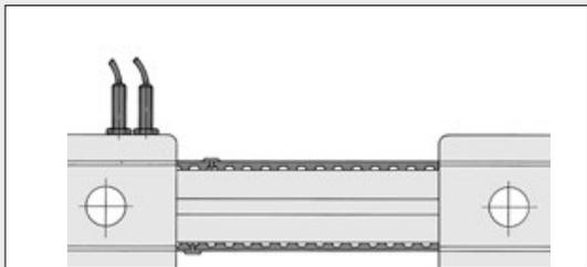
Possible arrangement of Proximity Switches 8 and Proximity-Switch Cams 8:
