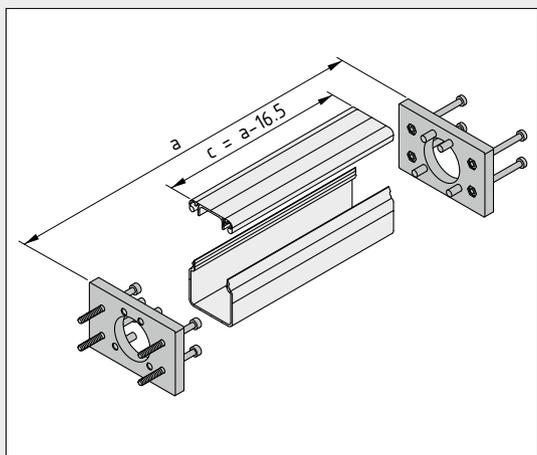
The adapter plates included in the Synchroniser Shaft Cover Set secure the conduit elements between the two timing-belt drives of Linear Units GSF 8 40 R10. Calculating the length:
