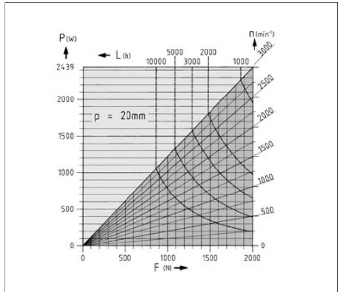
The service life of the screw and drive nut combination can be calculated based on the thrust load and drive speeds
